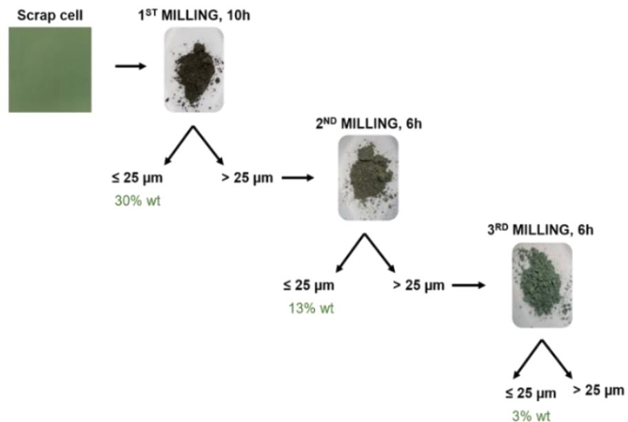
Figure 18 SOFC scrap cells EoL milling and sieving steps
