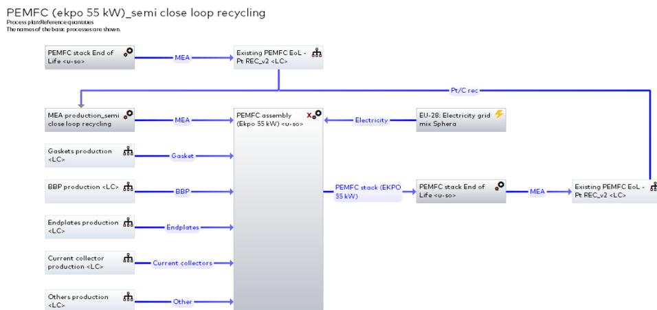
Figure 24: Semi close-loop LCA model for existing Pt recycling.
