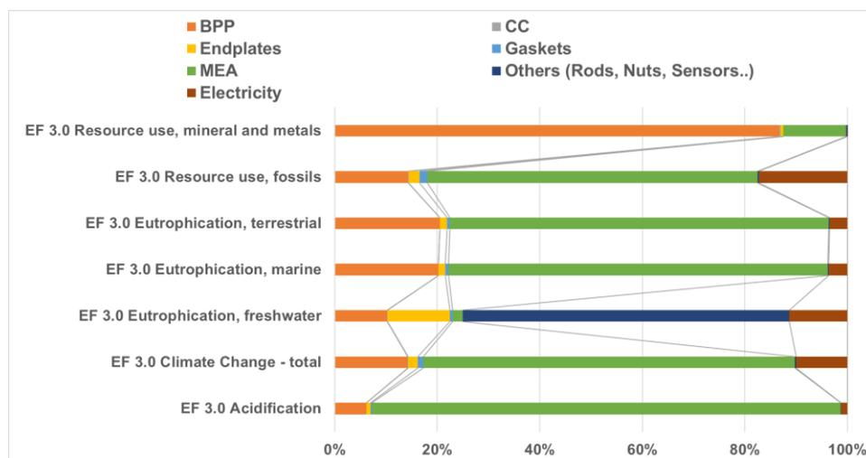
Figure 20 The main components and electricity contribution to the total environmental impact of the 55 kW<sub>el</sub> PEMFC stack
