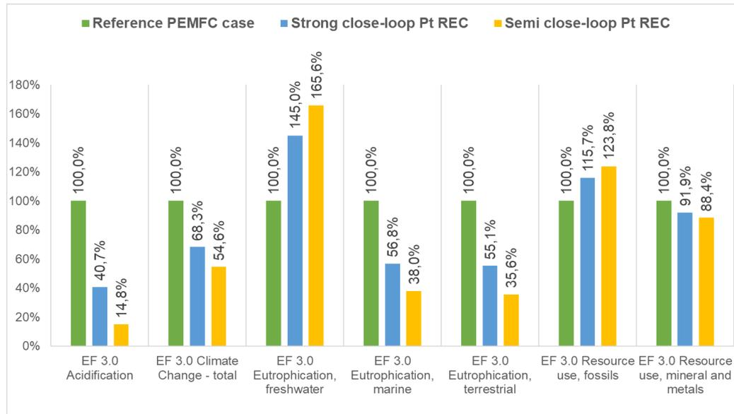
Figure 25: The relative effect and comparison of existing BEST4Hy EoL technologies (Pt REC) with different EoL scenarios for the manufacturing phase of 55 kW PEMFC stack.
