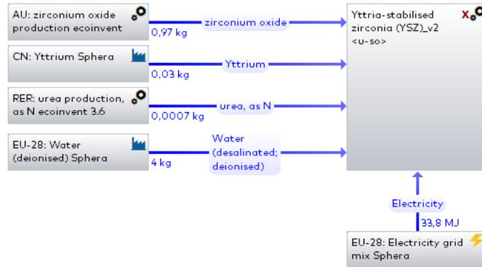
Figure 12 LCA model used for yttria-stabilized zirconia (3YSZ)
