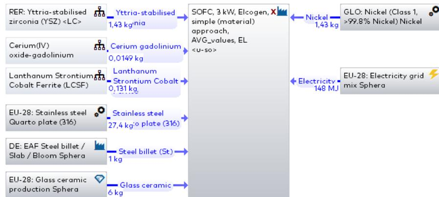
Figure 13 LCA model for manufacturing phase of the 3kW<sub>el</sub> SOFC stack
