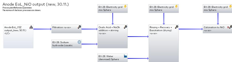
Figure 17 LCA model for NiO recovery from aged SOFC anode
