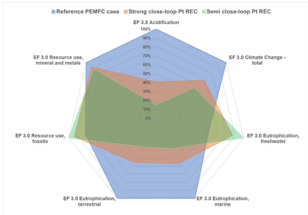
Figure 26: The relative comparison of different EoL scenarios (Pt recycling) effect on manufacturing phase of 55 kW PEMFC stack
