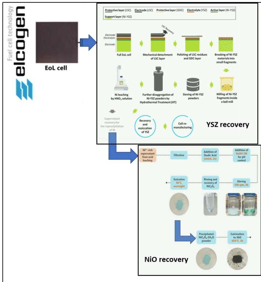
Figure 14 Existing SOFC EoL – YSZ and NiO recovery processes workflow
