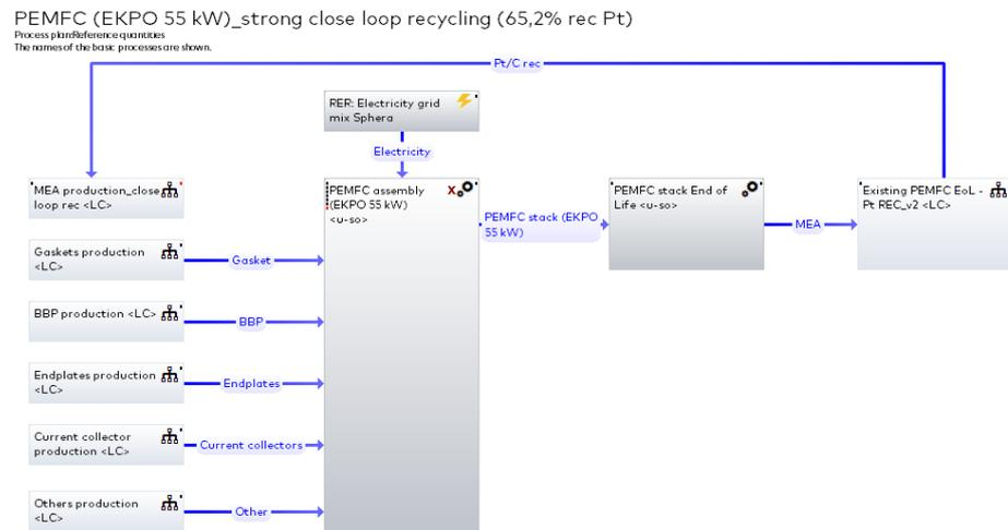
Figure 23: Strong close-loop LCA model for existing Pt recycling.
