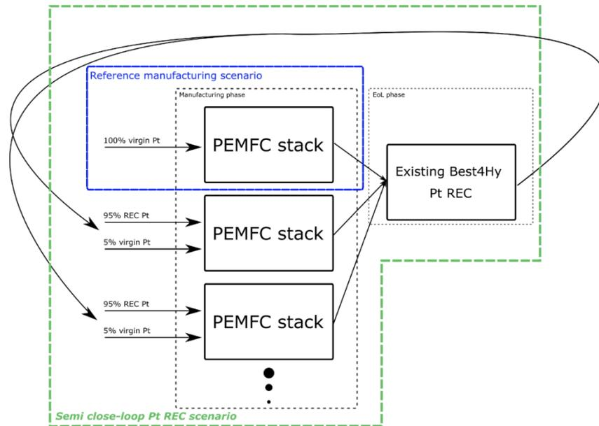
Figure 11: PEMFC semi close-loop Pt REC scenario.
