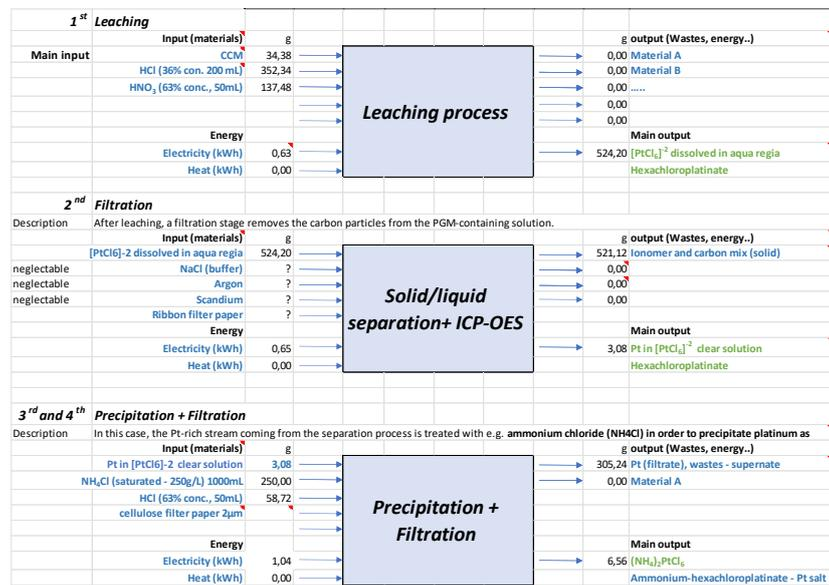
Figure 7: Hydrometallurgical treatment steps with energy and mass balances.
