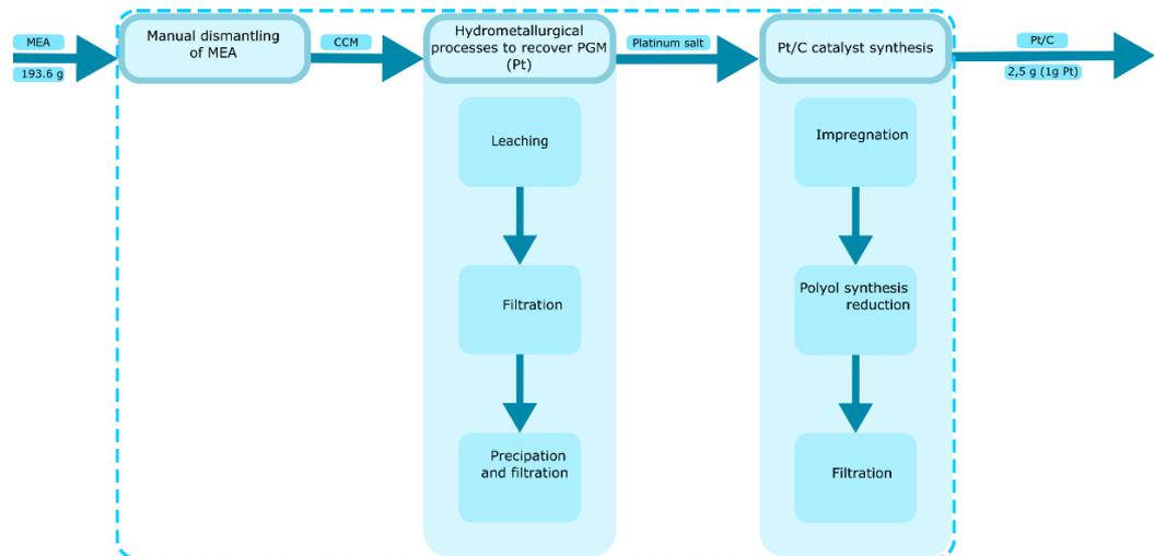
Figure 5 Existing PEMFC EoL – Pt recovery workflow
