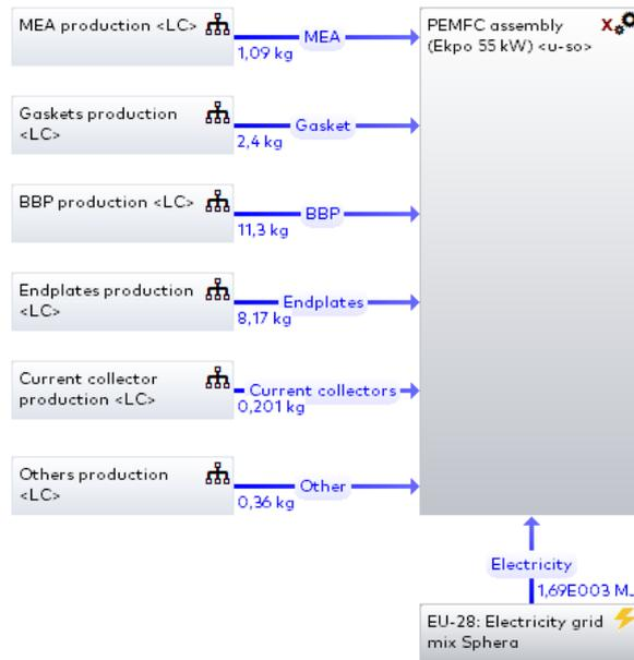
Figure 4 LCA model for manufacturing phase of reference 55 kW PEMFC stack
