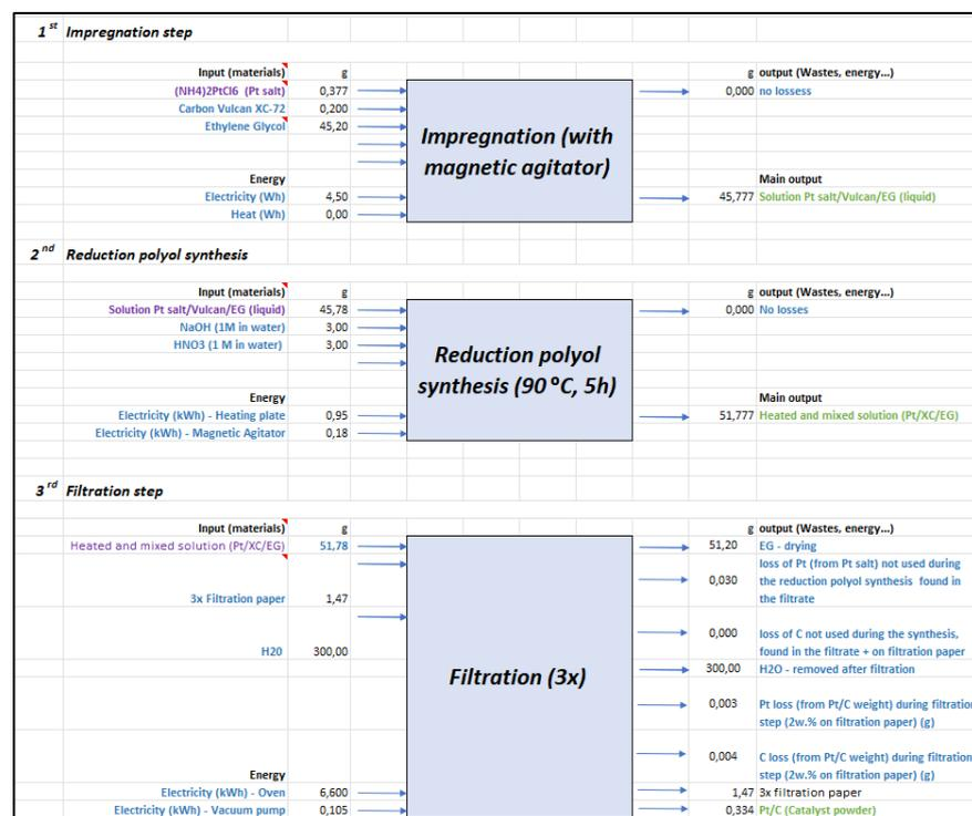
Figure 8: Pt/C catalyst synthesis steps with energy and mass balances.
