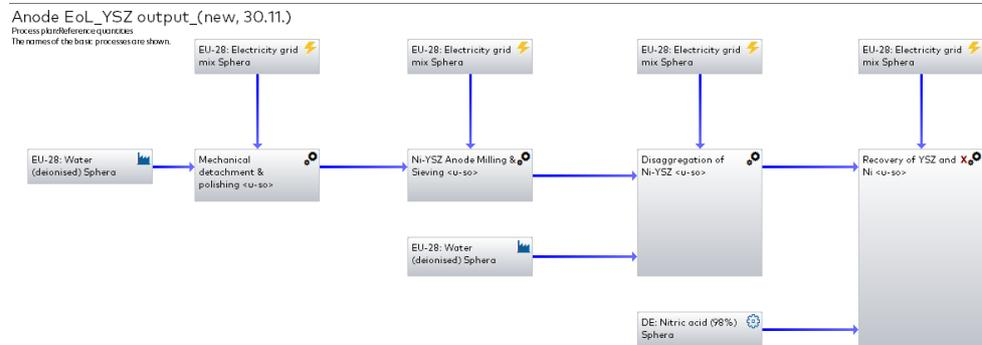
Figure 16 LCA model for YSZ recovery from aged SOFC anode
