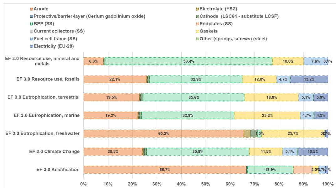
Figure 27: The relative contribution of each SOFC stack component and electricity to the total environmental impact of 3kW<sub>el</sub> SOFC stack
