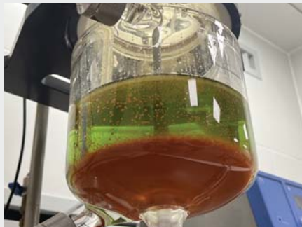
Three-step process for the extraction of platinum from EoL PEMFC (CCM component) and the production of Pt salt as the recovered product. Shown from left to right: leaching, precipitation, and Pt salt.
