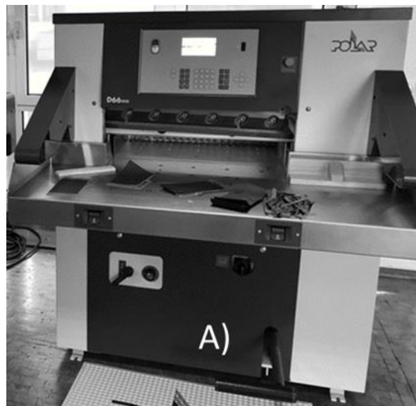
Figure 14 Polar equipment used to dismantle MEA units
