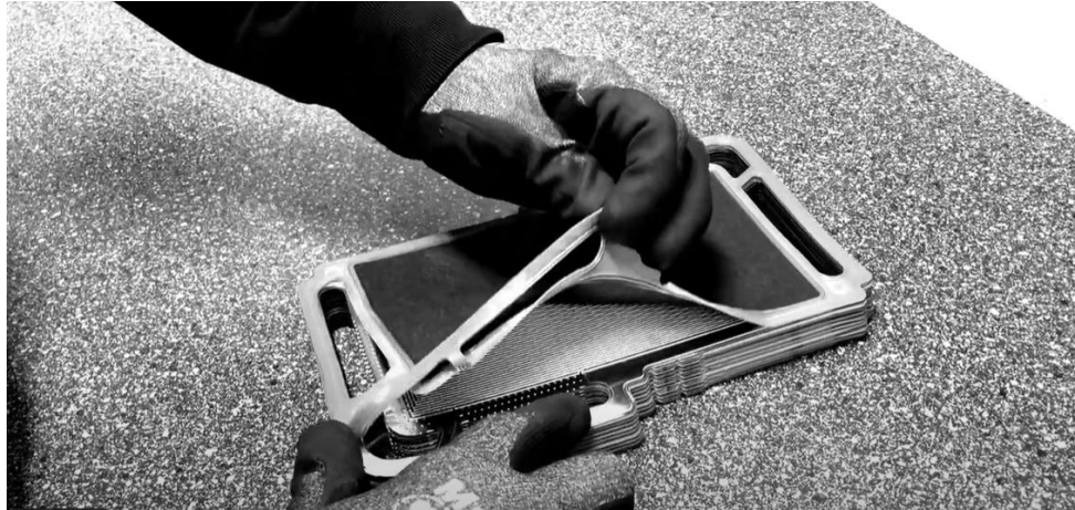
Figure 4 STEP 1: Separation of the bipolar plate from the MEA manually
