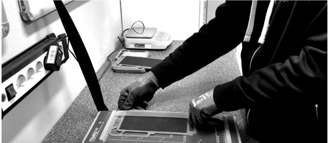
Figure 6 STEP 2: Cutting of rubber sealant by means of a lever cutting machine
