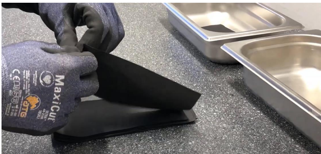
Figure 8 STEP 3: Manual separation of the CCM from the GDL
