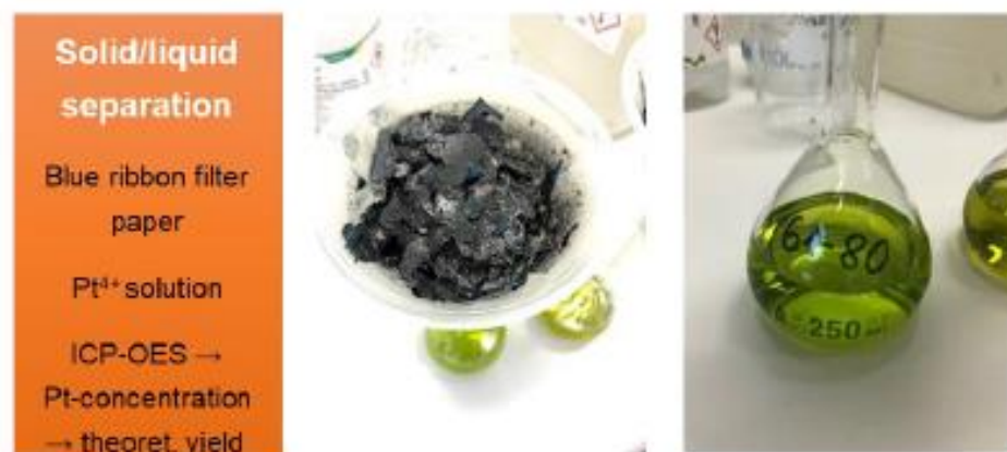
Figure 3 Solid/liquid separation step - BEST4Hy tests and samples
