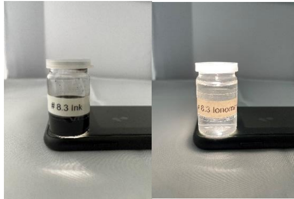
Figure 7 Example of separated fraction, Ionomer and Pt ink
