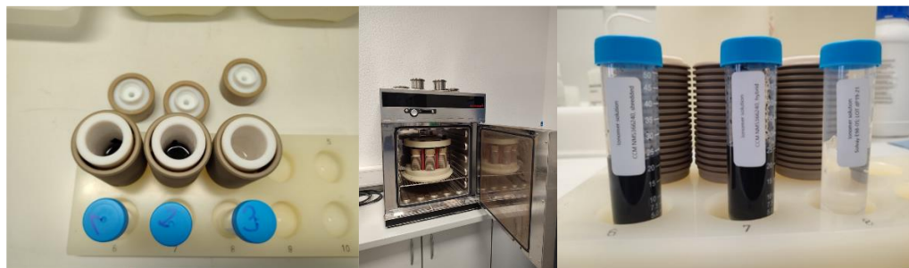
Figure 6 Dissolution tests using pressure vessels.
