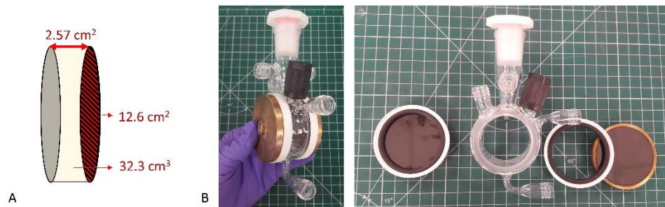
Figure 3 Dimensions of the improved electrochemical vessel (A) and pictures of the vessel (B)
