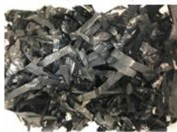
*Figure 4: Freshly shredded CCM material*
