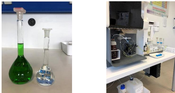
Figure 10: Pt rich solution and 1:100 dissolution ready for ICP-OES
