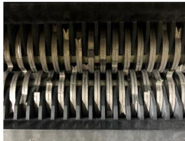
*Figure 3: Internal view of paper shredder with CCM fractions traces*
