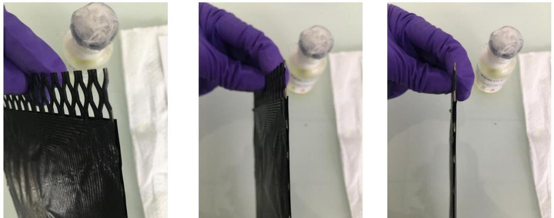
Figure 33: photographs from different angles of a DSA with CCM on both sides
