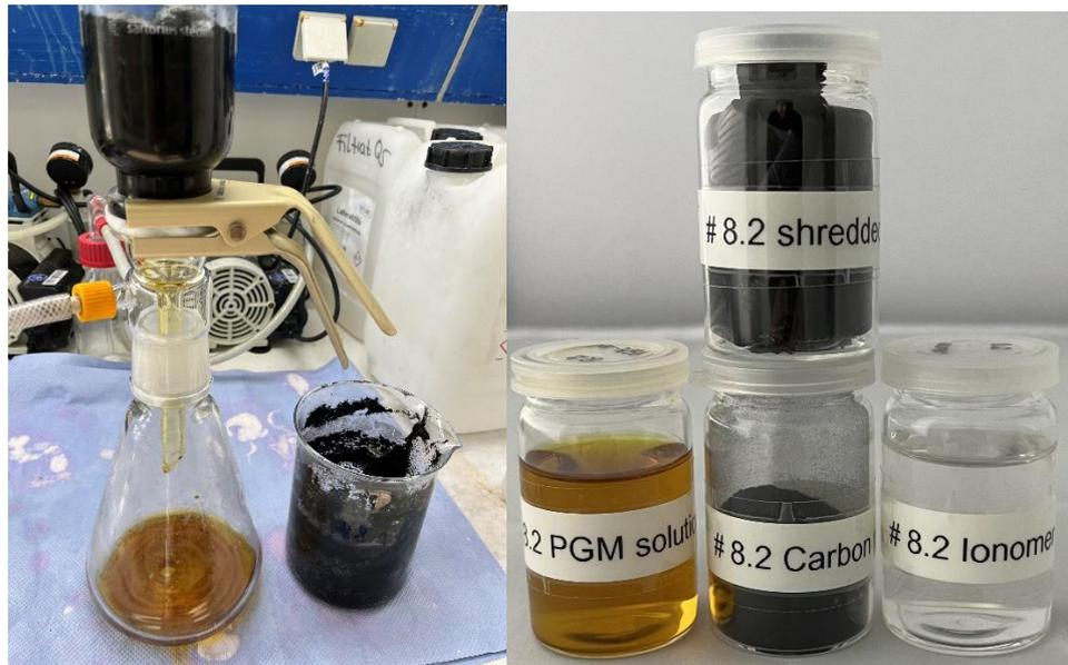
Figure 26 HMT route of recovered PGM ink from AD process and final products, showing the initial material (CCM), PGM solution, ionomer solution and recovered carbon from CCM)
