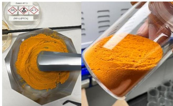
Figure 6: recovered Pt as ammonia hexachloroplatinate from batch #7.3
