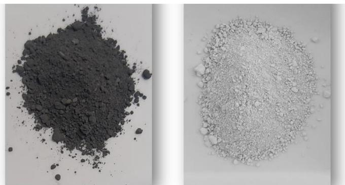
Figure 11 Visual aspect of the powders recovered (left) after acidic leaching carried out in the reactor at the laboratory-scale, (right) after acidic leaching carried out in the pilot-scale reactor at TRL5 (200 °C, HNO<sub>3</sub> 1.0 M, stirring 650 rpm) (c).
