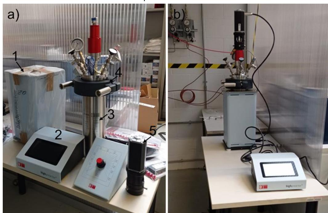
Figure 3: Reactor components (a) before the installation. Reactor system after the installation (b) ready to use.
