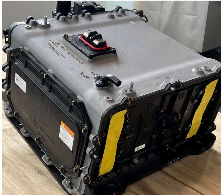
Figure 3. Whole stack coming from an EOL hydrogen passenger car (M1).
