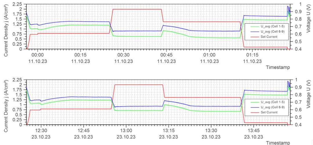
Figure 6: PHT after break-in procedure (top diagram, after ~7.5 operating hours) and PHT at end-of-test (bottom diagram, after ~200 operating hours).
