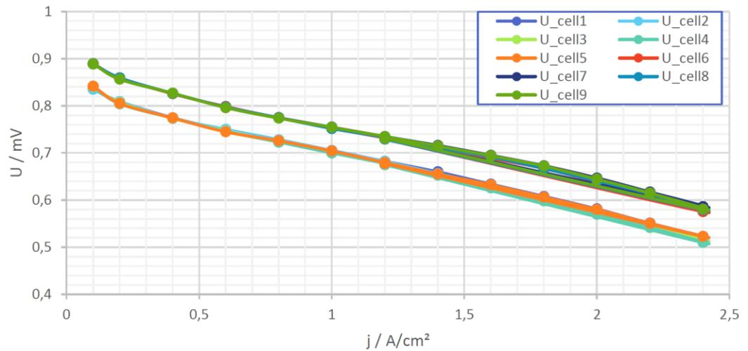
Figure 8: one exemplary polarization curve from short stack testing displaying single cells, B4HyCCMs being constantly lower in voltage. Operating parameters to be found in the annex (Table of Operating Parameters of exemplary polarization curve).
