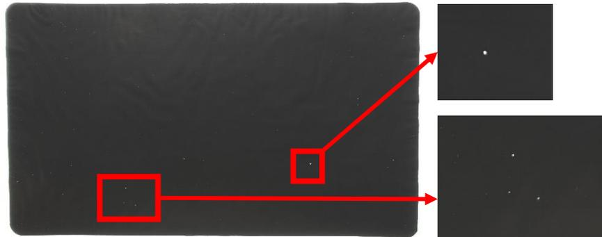
Figure 4: spots with no coverage of catalyst layer on both sides of BEST4Hy CCMs
