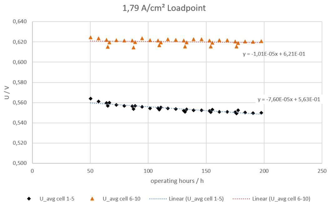
Figure 11: Evaluation of 1.79 A/cm<sup>2</sup> load point of durability load cycle
