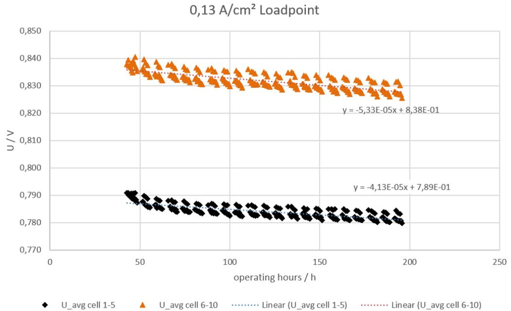
Figure 14: Evaluation of 0,13 A/cm<sup>2</sup> load point of durability load cycle
