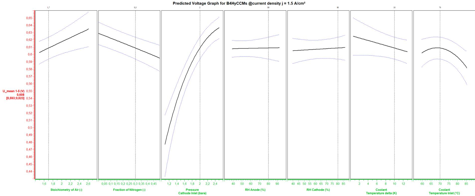
Figure 10: Predicted response graph for the averaged cell voltages of cells containing B4HYCCMs in reference to different factors. Factors fixed to one exemplary operating point at a current density of  $1.5 \text{ A/cm}^2$ .
