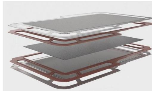
Figure 3: EKPO NM5 cell concept with BPPs, seals and MEA (GDLs and CCM). The seals, which appear separated here, are however injection molded onto the GDLs
