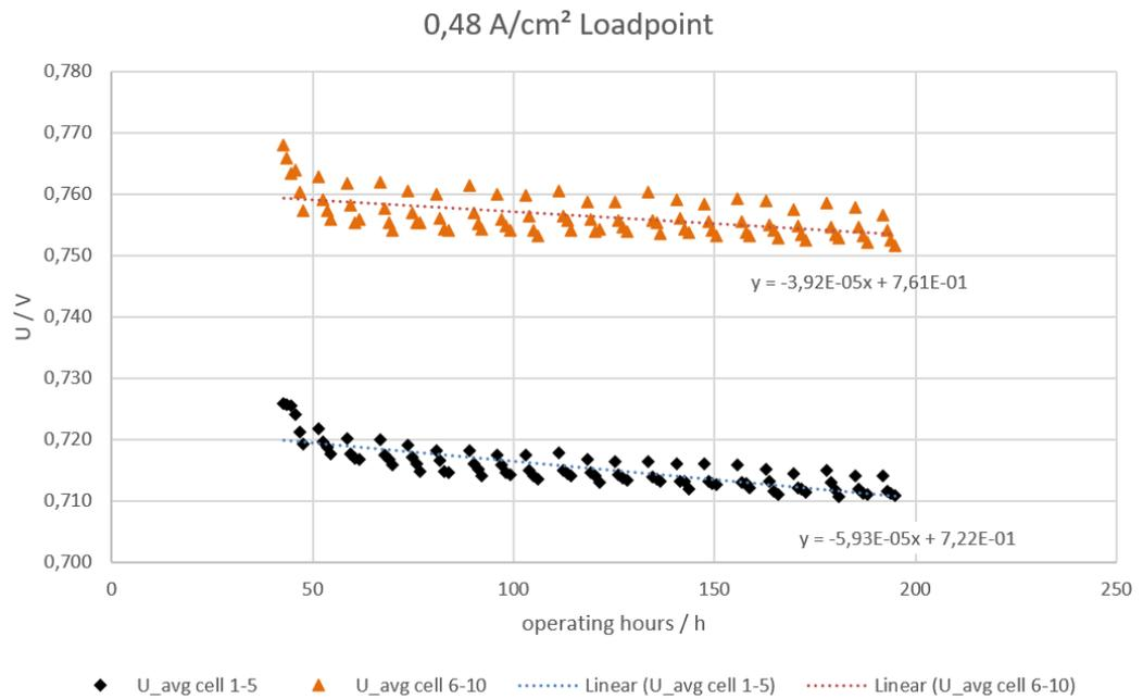
Figure 13: Evaluation of 0,48 A/cm<sup>2</sup> load point of durability load cycle
