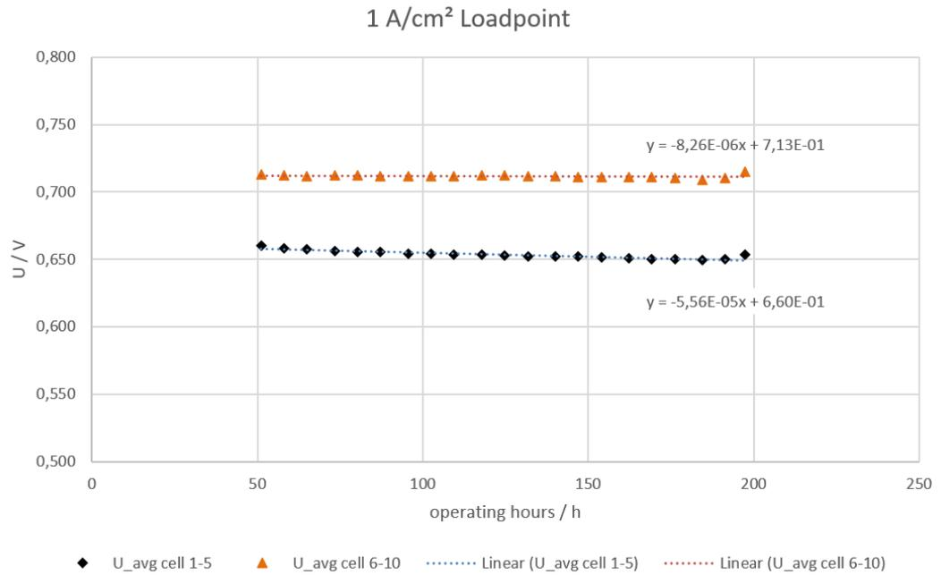
Figure 12: Evaluation of 1 A/cm<sup>2</sup> load point of durability load cycle
