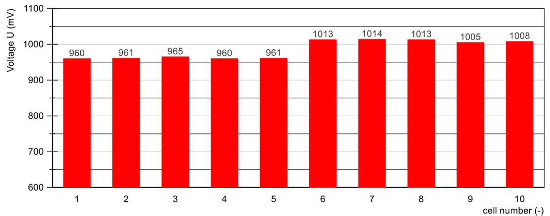
Figure 9: Open circuit voltage of short stack single cells with B4HyCCMs (1 to5) and RefCCMs (6-10).
