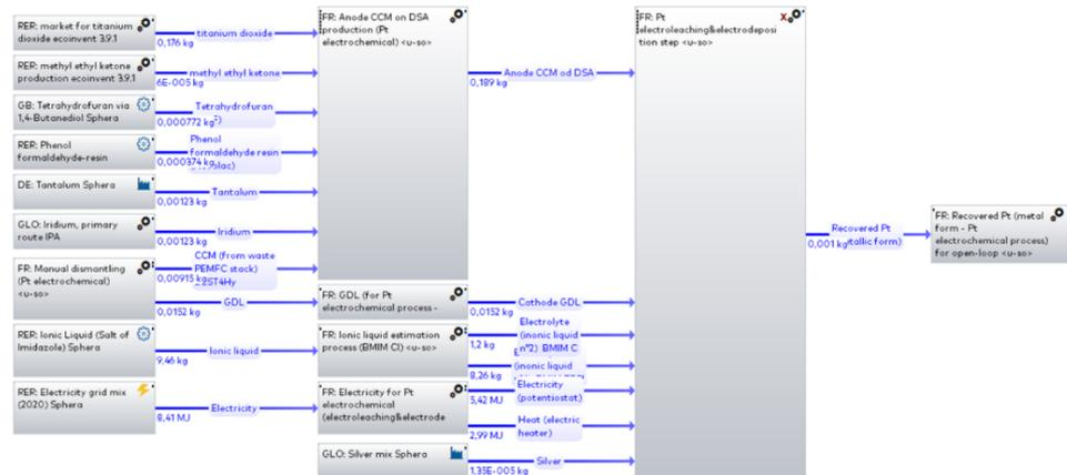
Figure 4: LCA model for BEST4Hy Pt electrochemical recovery process
